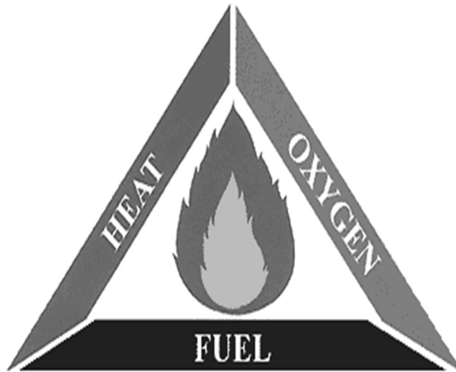
The Triangle of combustion
